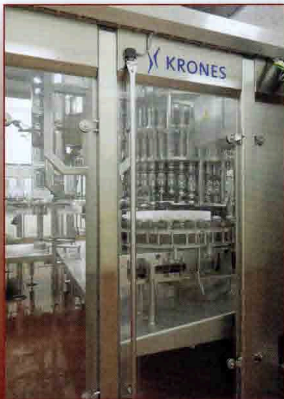
Newly sterilized bottles pass through a bottle filler in Dr Pepper Snapple Group's facility in Victorville, Calif.
